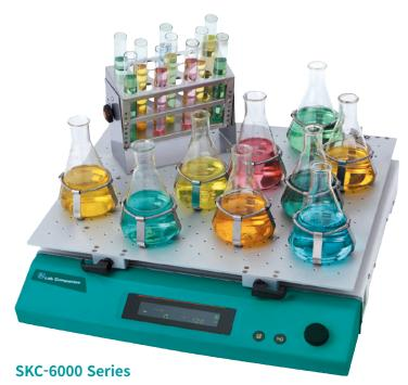
with Universal Platform, Flask Clamp, Test Tube Rack (Option)
