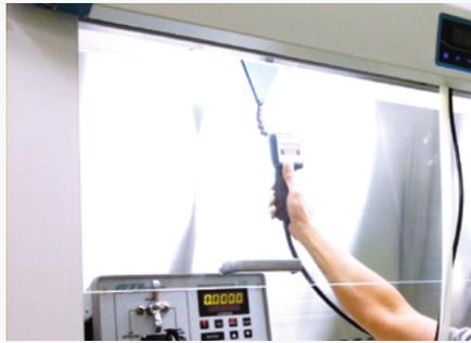
HEPA Filter Leak Test
